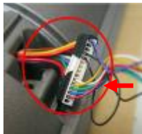
System connector supports PS/2 and RS-232 interface
